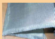
Figure 4. Woven glass filament (E-glass and steel wire)
