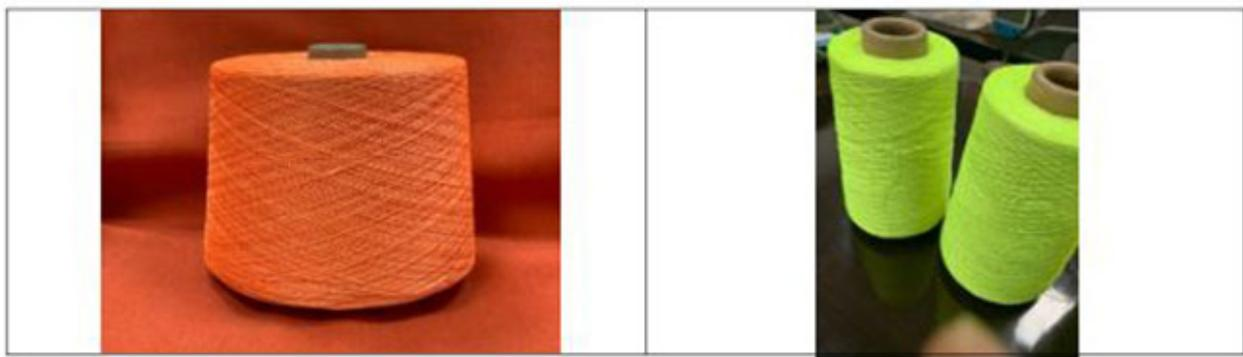
Figure 3. HPPE in core with Hi-vis nylon orange and green on sheath
