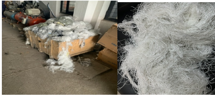
Figure 1. Spinning waste of High Performance Polyethylene Fibres (UHMWPE) twisted with 50 micron of stainless steel
