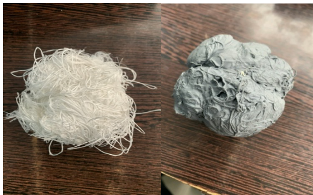
Figure 5. Spherical structure created using metallic waste yarns of UHMWPE
