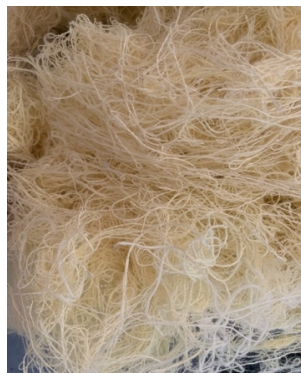
Figure 2. Metallic Aramid yarn waste generated during automatic clearing & winding
